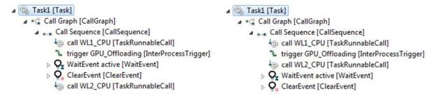
Figure 11: Synchronous offloading (left) and asynchronous offloading (right)
